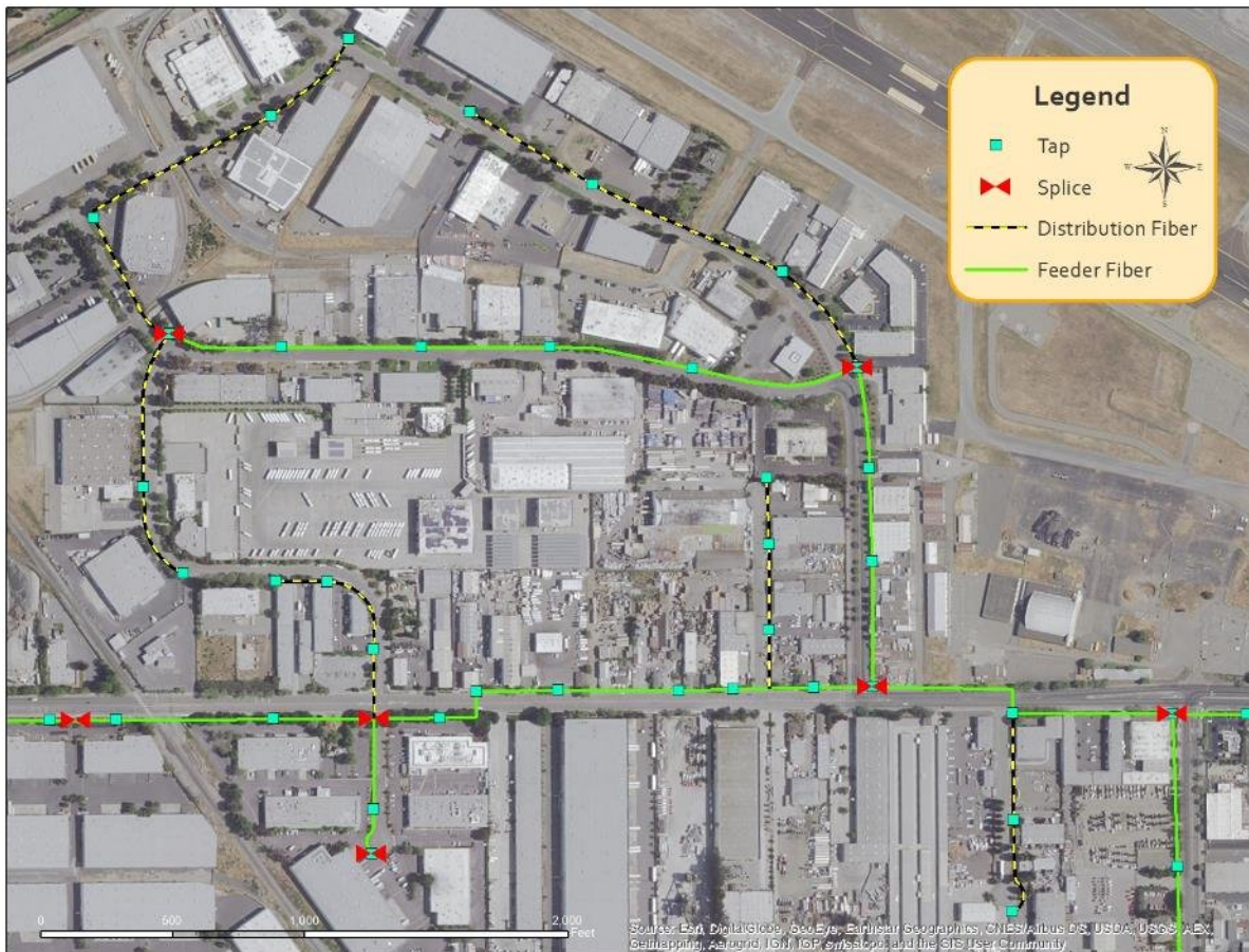
Figure 6: Detail Showing FTTP Access Layer Design
