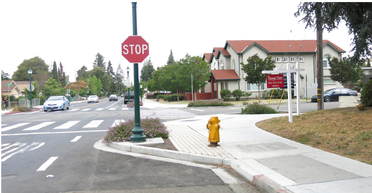
Corner bulbouts on Dixon Street and Valle Vista Avenue.
