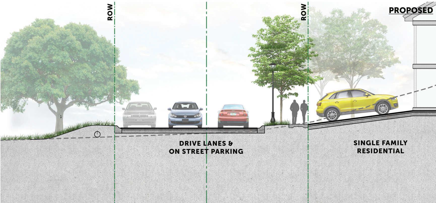
Figure 4-8: Maitland Drive Proposed Development Typical Street Section
