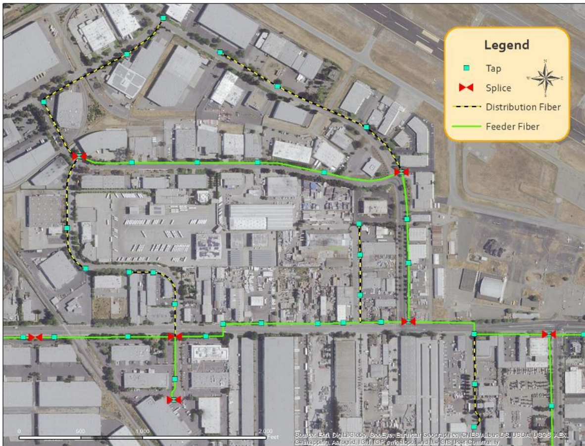
Figure 6: Detail Showing FTTP Access Layer Design
