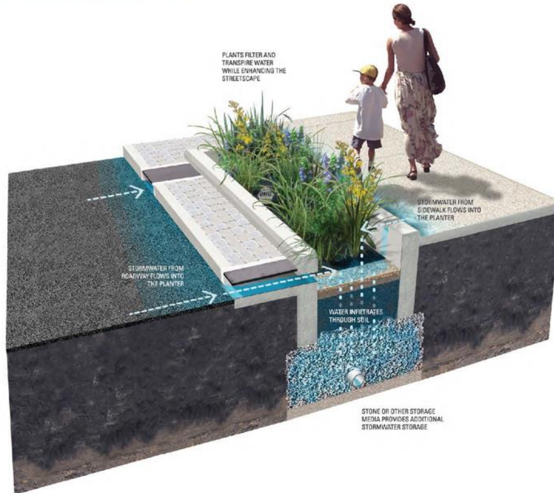
Figure 2.1: Three-Dimensional View of a Stormwater Planter
