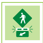
Rectangular Rapid Flashing Beacon
