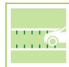
Painted Optical Speed Bars
