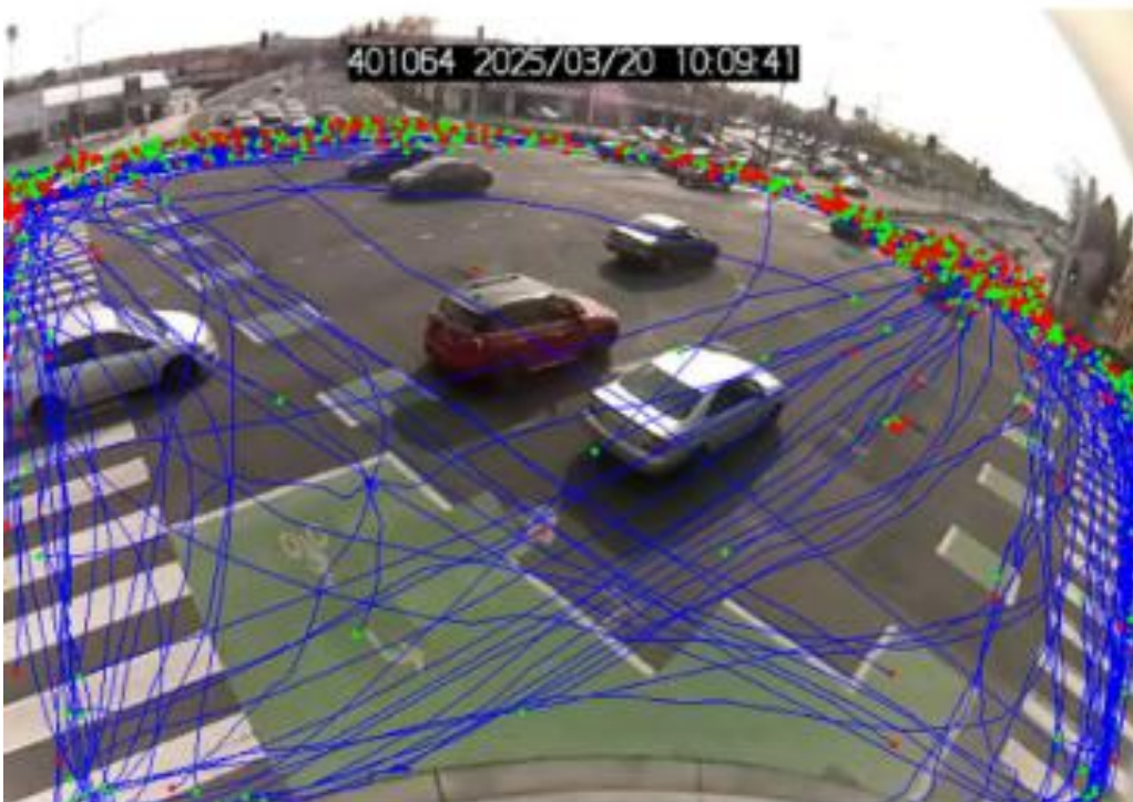
Figure 1: Weekday bicycle path of travel at Hesperian Blvd & West A St (looking southeast).
