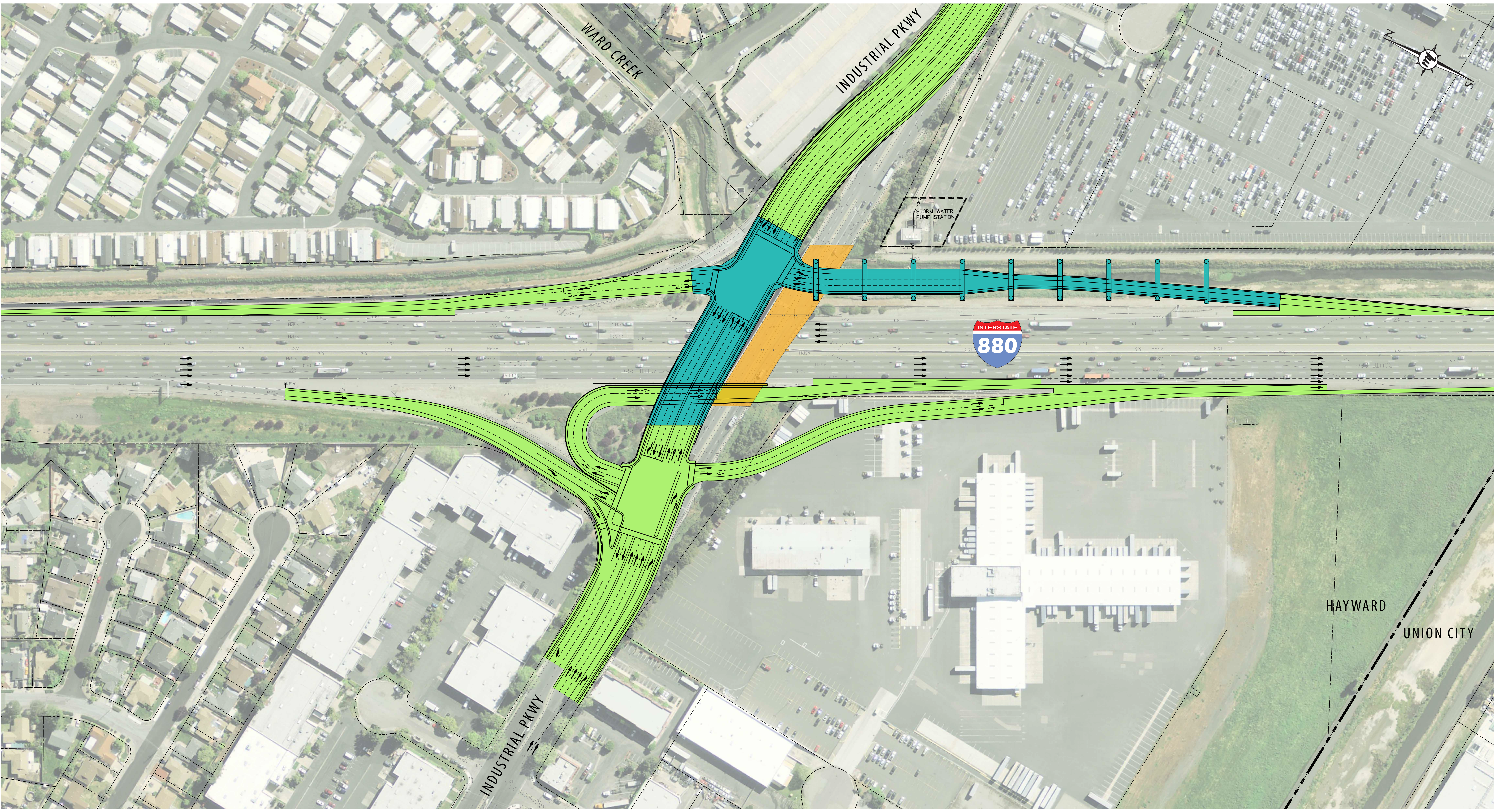
INDUSTRIAL PARKWAY ALTERNATIVE 3 NB L-1 TIGHT DIAMOND SB L-9 LOOP & TIGHT DIAMOND
