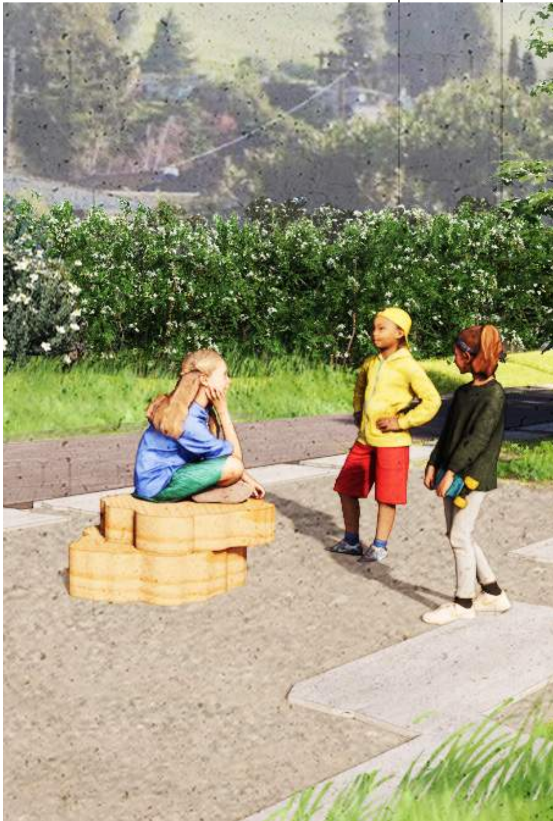
Tree Cookie Seating Element Detail - 25 Available Segments: 24-36" Diameter, 6-24" Lengths
