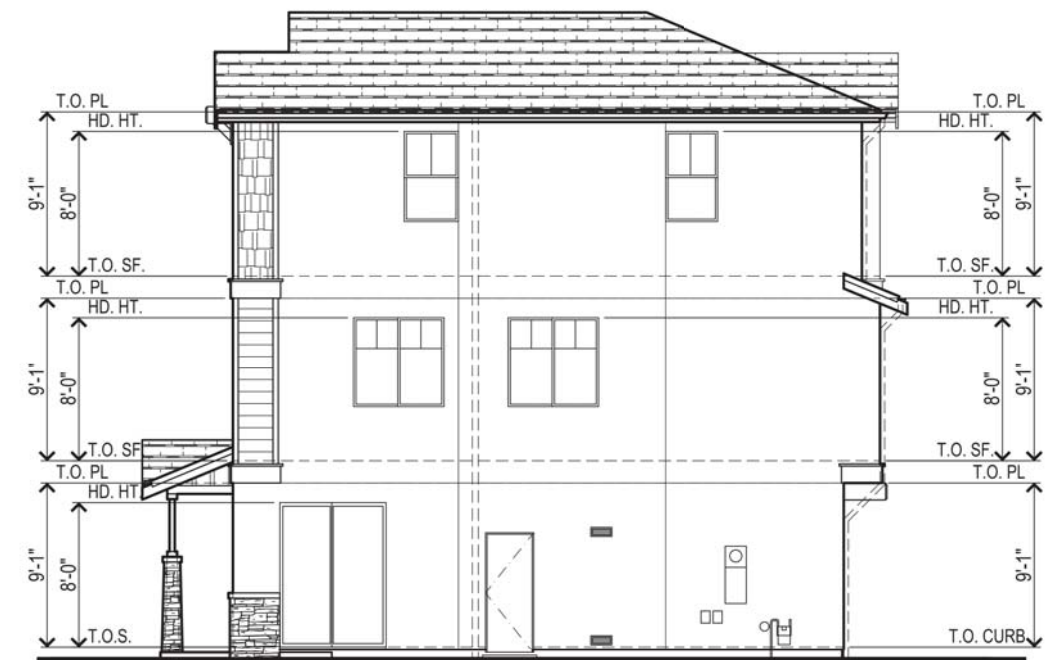
CRAFTSMAN 'B' RIGHT ELEVATION SCALE: 3/16" = 1'-0"
