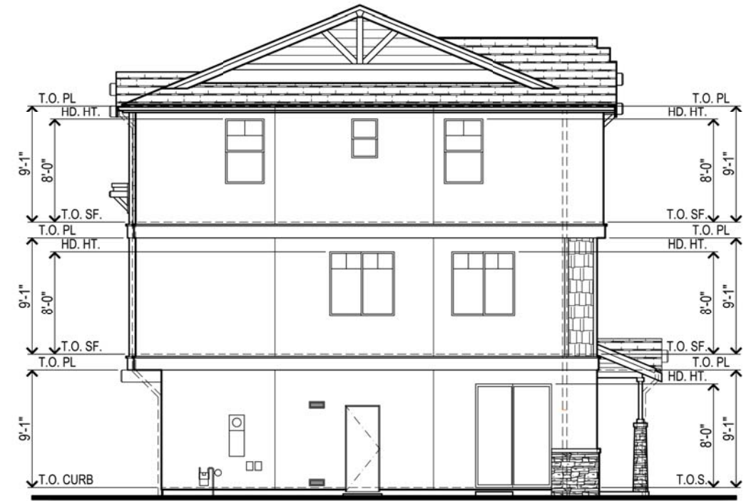
CRAFTSMAN 'B' LEFT ELEVATION SCALE: 3/16" = 1'-0"
