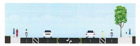
Restriping is proposed to help reduced speeds, which often exceed 45 mph. The proposed restriping includes one lane in each direction, with a buffer in the westbound (downhill) direction and separation in the eastbound (uphill) direction.
