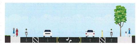
Restriping is proposed to help reduced speeds, which often exceed 45 mph. The proposed restriping includes one lane in each direction, with a buffer in the westbound (downhill) direction and separation in the eastbound (uphill) direction.
