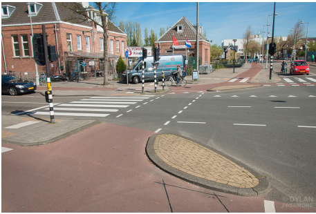
Protected intersection with colored pavement
