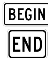
Figure 4 Optional signage for the start and end of bike lanes
