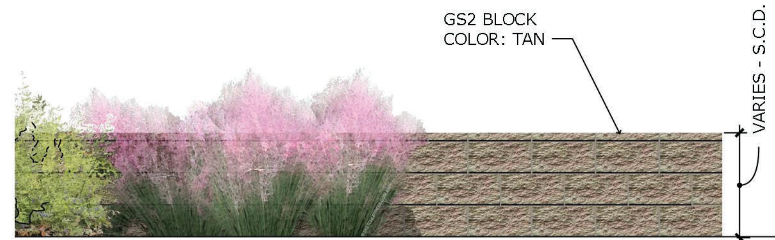
A RETAINING WALL 6 scale: 1/2"=1'
