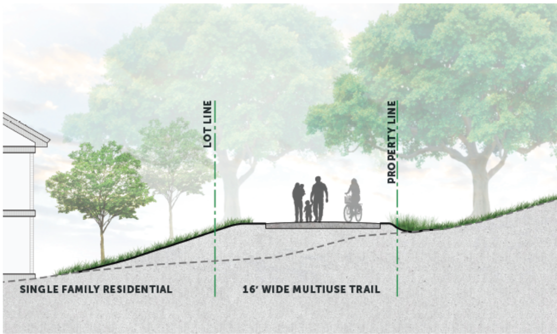
PROPOSED CONDITION - GRADED SLOPE
