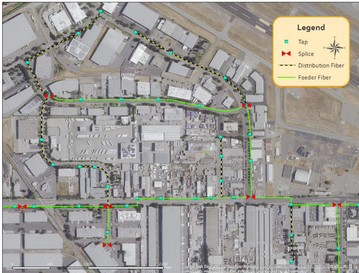
Figure 6: Detail Showing FTTTP Access Layer Design
