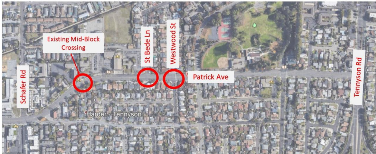
Figure A: Proposed RRFBs at the intersections of Patrick Avenue and St. Bede Lane, and Patrick Avenue and Westwood Street, and mid-block between intersections of Patrick Avenue and Schafer Road, and Patrick Avenue and St Bede Lane
