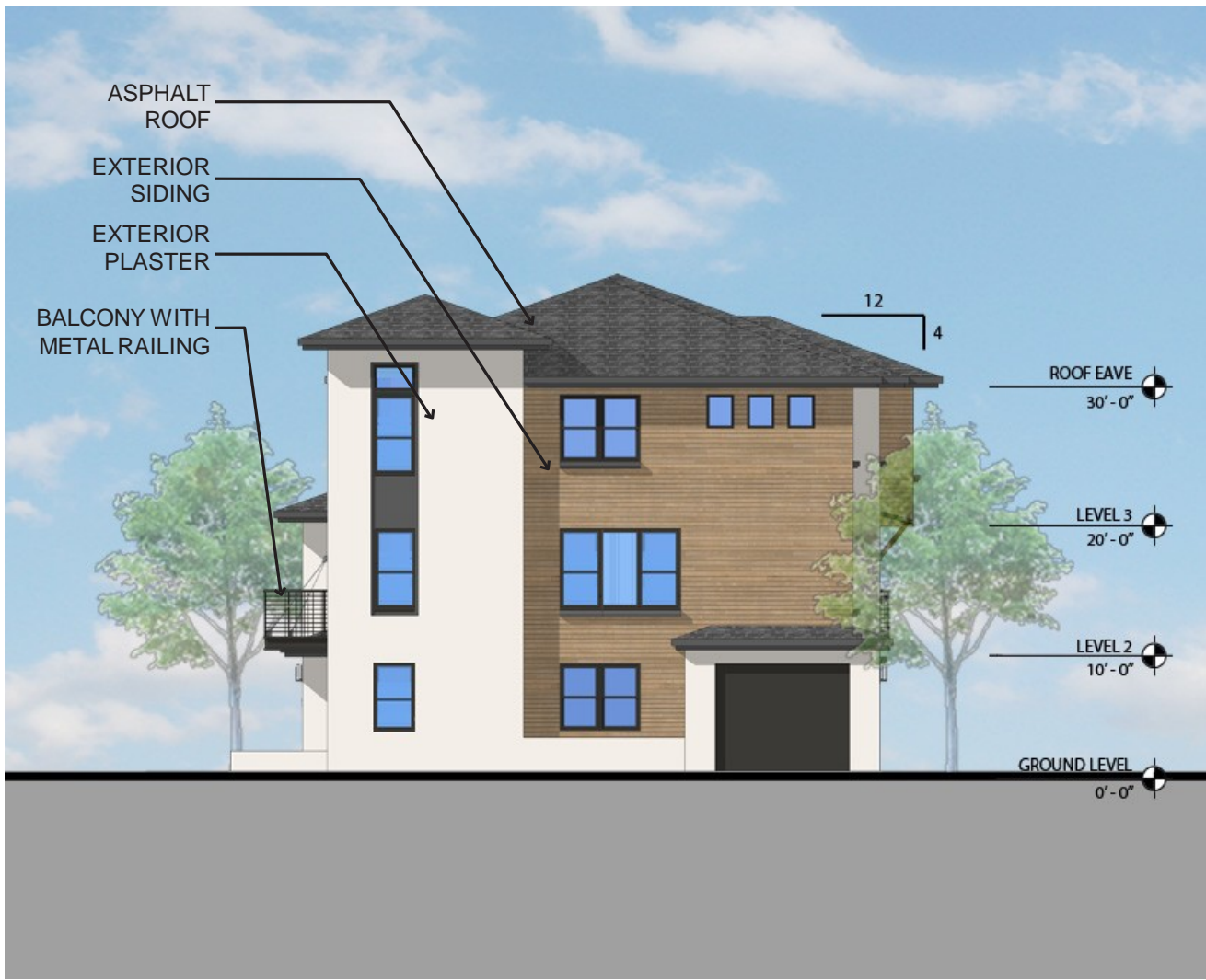
Building 4A - Right Elevation SCALE: 3/16" = 1'-0" 3
