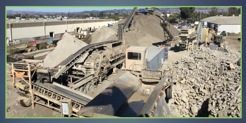
Noise Study prepared for the Depot Site recommends that the crusher should be at least 100 feet from the property line to be under 70 dba.
