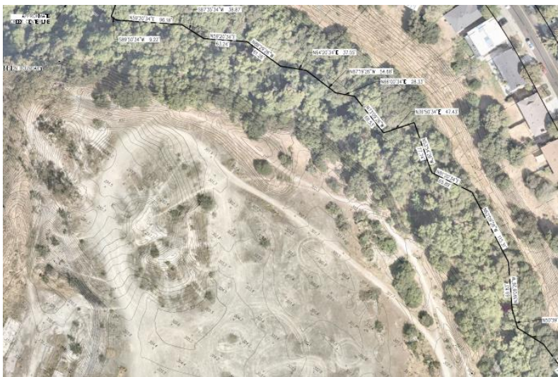
Excerpt of Rose Hills Sheet 2 existing site conditions showing top-of-bank areas largely scraped clean of vegetation and topsoil.
