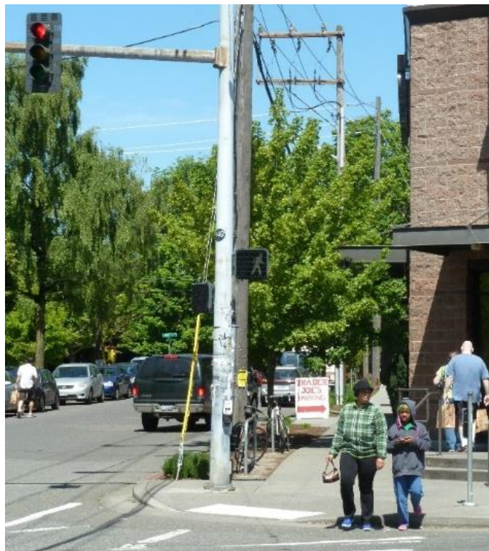
Example LPI with WALK signal during red signal phase. Source: Kittelson & Associates, Inc
