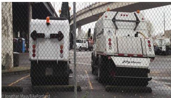
Example of a smaller street sweeper for separated bikeways and trails next to a standard size street sweeper.
