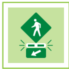
Rectangular Rapid Flashing Beacon
