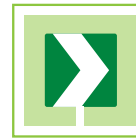
Chevron Signs on Horizontal Curves
